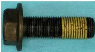
ZOH-T Bolt: flange head, dark in color, fine thread, may have thread patch as shown (M12x1.25x40).
